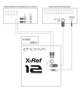
A typical installation, with a single X-Ref 12 DSP Powered Subwoofer providing bass enhancement for both a stereo system and a home-theater pre/processor
